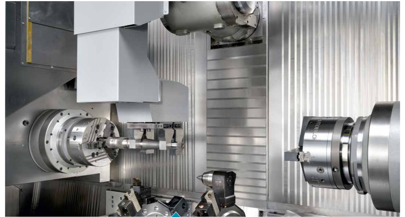
Removal of finished parts (or feeding) using a workpiece-specific gripper for shaft parts or flange parts
