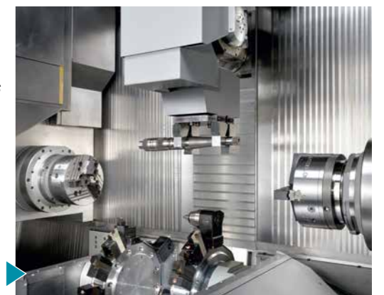
2-axis workpiece handling system moves to the removal point without collision
