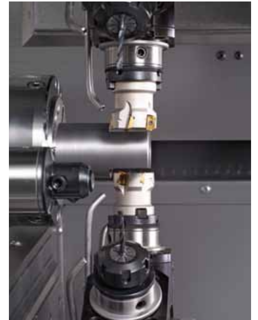
Y functionality on both tool turrets: Milling of surfaces (Y-travel +/- 50 mm)
