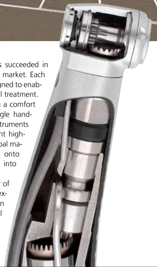
Each component in the mechanically-driven contra-angle handpiece requires maximum precision in order for the tool to ultimately achieve 200,000 rpm and have a long service life. Figure: W&H
